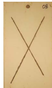
Bonderite 1000 / Parcolene 60 Iron Phosphate w/chrome seal
